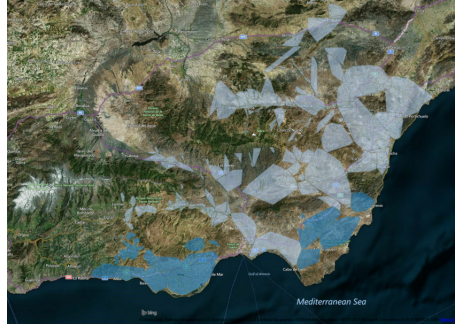
Fig. 3: GIS visualization of the STUMP (the blue areas mark the WMAs with higher consumption of water per hectare Campo de Nijar and Poniente compared to the gray ones).
